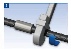
Tighten the joint using a wrench on the continuation bar. After tightening there should be no more than 2-4mm of thread exposed, depending on the diameter of the rebar.
