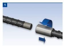
Screw the coupler to the rear of the thread on the continuation bar.
