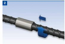
Remove the plastic cap from the coupler. Position and rotate the continuation bar in the coupler.
