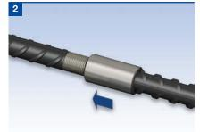
Position the continuation bar with the coupler against the end of the first bar.
