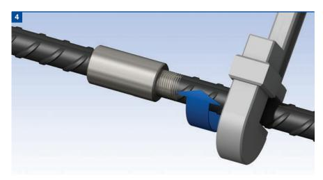
Using a wrench, rotate the continuation bar to lock the two bar ends against each other within the coupler. After tightening, the length of exposed thread should be no more than half of the coupler length plus 2-4mm depending on the diameter of the rebar.
