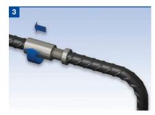
Rotate the coupler from the continuation bar to engage against the rear of the thread on the opposing bar and lock tight.
