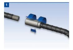
Screw the locknut followed by the coupler to the rear of the thread on the continuation bar.
