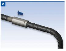
Position the continuation bar with the coupler against the end of the first bar.
