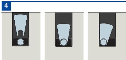
After a predetermined time period (generally 3-4 weeks), when movement between the slabs has stabilised and the joint between the slabs has been filled, the dowel is ready to be locked.
