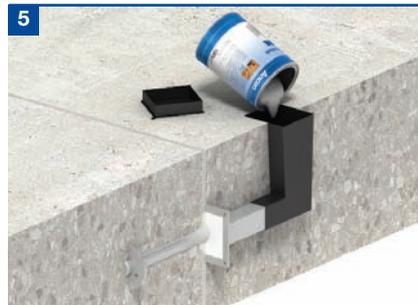
Mix the two-part epoxy resin and pour into the void former. It is essential the resin flows along the stainless steel box section towards the joint and reaches the notches on the locking plate, which indicate minimum resin depth. Joint must be filled before resin is installed.
