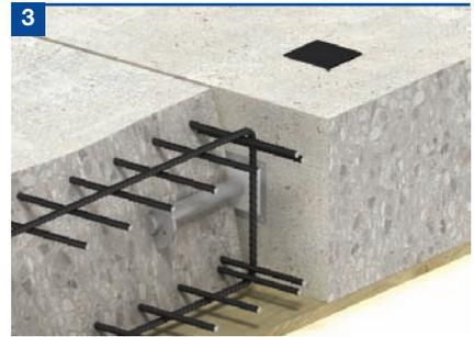
Fix the local reinforcement around the dowel component and pour the concrete.
