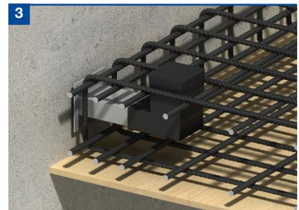
Puncture the label of the sleeve to reveal the cylindrical sleeve only. Push the sleeve over the dowel until it is flush with the concrete. Tie the sleeve to reinforcement and pour concrete.
