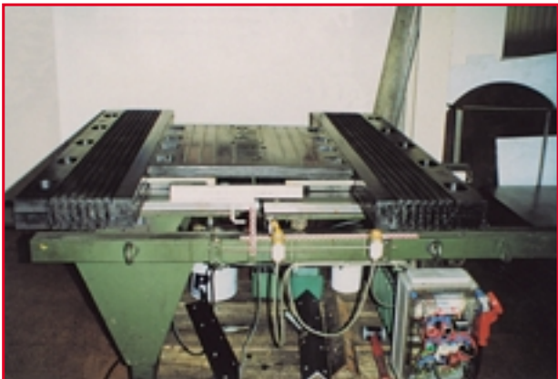
Expansion joint being tested at FIP laboratory
